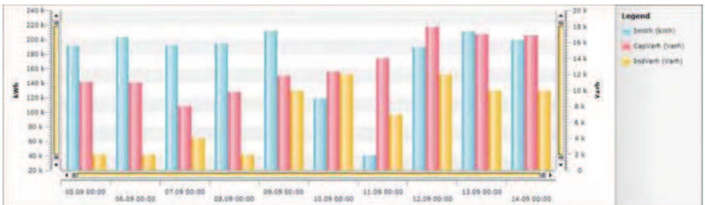
Active and reactive energy consumption of a PFC panel throughout 10 days
