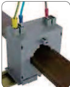
Connect the cable S1 in one of the two terminals of the corresponding side, and the cable S2 in one of the two cables of the opposite side. The selected terminal is irrelevant since the two adjacent Fast-On terminals are internally connected. The cable / bar of the primary current must be inserted into the transformer paying attention to the flow direction of the current, which must always be in the direction P1 → P2.
