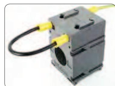
The double terminal lets you make a short-circuit when it is necessary to disconnect the load from the transformer, so as not to damage the transformer or the operator. It is also possible to ground it if you do not want to use the same terminal used for connection to the load.
