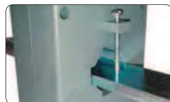
Fixing possible for all codes, using the two screws supplied with the transformers, as shown in the figure. In this case, be sure to protect the tips to avoid the piercing of the primary cable.
