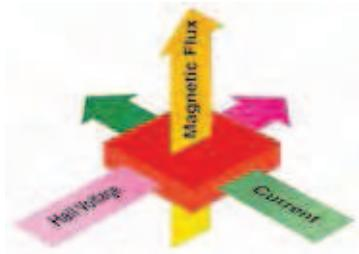
The function of the sensor is based on the "Hall effect" galvano-magnetic principle, named after the discovery of the American physicist Edwin Herbert Hall; namely the formation of a difference of potential on the opposite faces of the electrical conductor, due to a magnetic field perpendicular to the electric current that flows in it.
