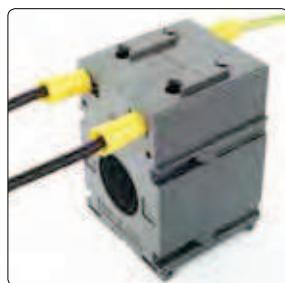
Connect the cable S1 in one of the two terminals of the corresponding side; and the cable S2 in one of the two terminals of the opposite side. The selected terminal is irrelevant since the two terminals in opposition are internally connected.
