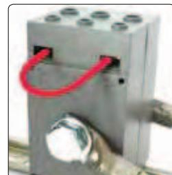
The double terminal lets you make a short-circuit when it is necessary to disconnect the load from the transformer, so as not to damage the transformer or the operator.
