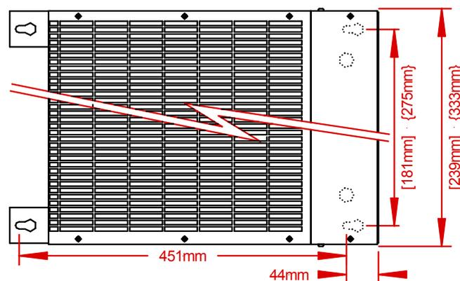
Unit is designed for mounting horizontally with the largest open face up. Other orientations may result in increased element temperatures. **Warning** - units must never be situated so that the terminal box is the highest point of the resistor. Units must never be situated so that the largest open face is at the bottom.
